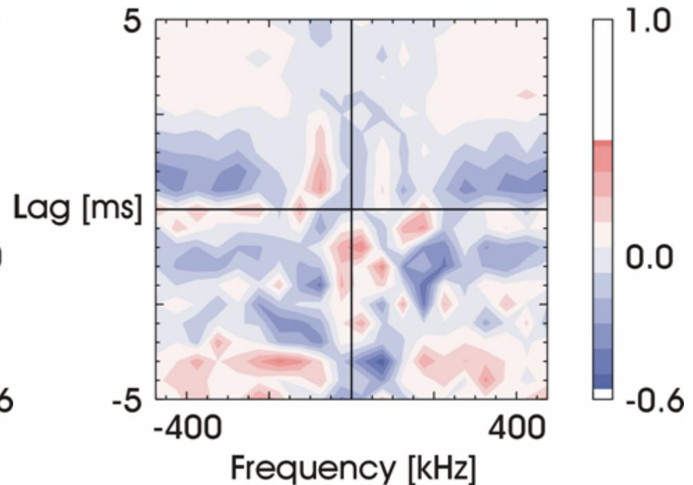
Positive (negative) time lag: Density fluctuations occur before (after) the magnetic fluctuations.
