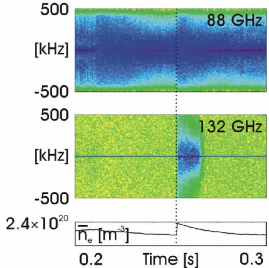
The 132 GHz signal disappears when the density decays below cutoff.
