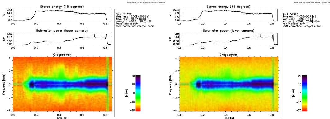
Figure 3: (Colour) Analysis of shot 51322, top to bottom: Stored energy, bolometer power and crosspower amplitude (logarithmic scale). Left: Slow time resolution (5 ms), right: Faster time resolution (1 ms).
