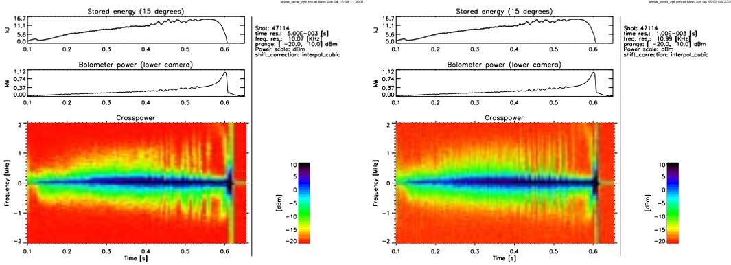
Figure 1: (Colour) Analysis of shot 47114, top to bottom: Stored energy, bolometer power and crosspower amplitude (logarithmic scale). Left: Slow time resolution (5 ms), right: Faster time resolution (1 ms).
