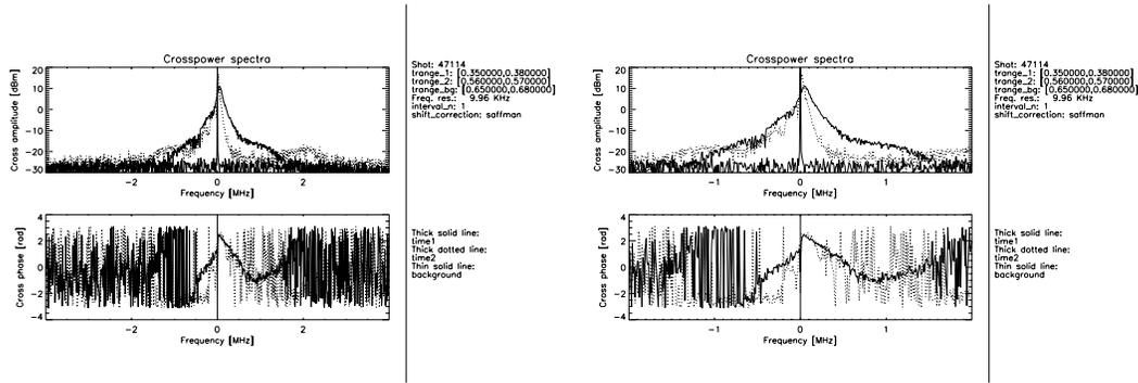
Figure 2: 2D plots of cross amplitude (top) and cross phase (bottom) between density fluctuations in the two volumes. Left-hand shows data up to  $\pm 4$  MHz, right-hand side up to  $\pm 2$  MHz. L-mode measurements are solid thick lines, H\*-mode measurements thick dotted lines.
