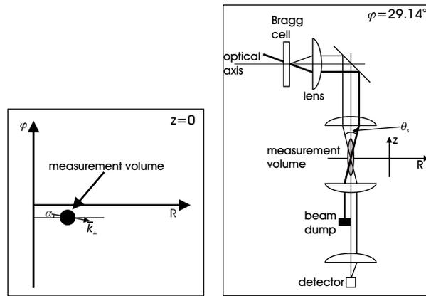
Figure 1: Left: View from above of the measurement volume created by two crossed beams having the same waist size, right: Side view of diagnostic setup. The M beam is the thick line and the LO beam is the thin line.
