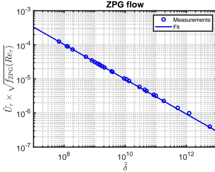
Figure 1: Correction term multiplied by dimensionless drag for ZPG flow as a function of  $\tilde{\delta}$ . Measurements from [1].
