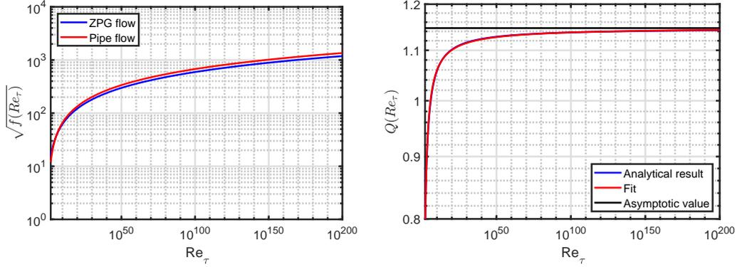
Figure 3: Note the extreme Reynolds number range, from  $10^2$  to  $10^{200}$ . Left-hand plot: Correction terms for ZPG and pipe flows as a function of  $Re_\tau$ , right-hand plot: Ratio of correction terms as a function of  $Re_\tau$ ; the horizontal black line indicates the asymptotic value of 1.15.
