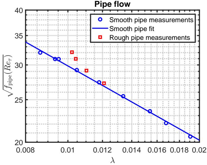
Figure 2: Correction term for pipe flow as a function of  $\lambda$ . Rough pipe measurements are shown for reference. Measurements from [7, 8].
