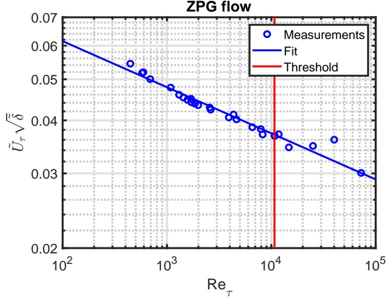
Figure 4: The product  $\tilde{U}_\tau \sqrt{\tilde{\delta}}$  as a function of  $Re_\tau$ . The vertical line at  $Re_\tau \sim 11000$  indicates the pipe flow transition found in [11]. Measurements from [1].
